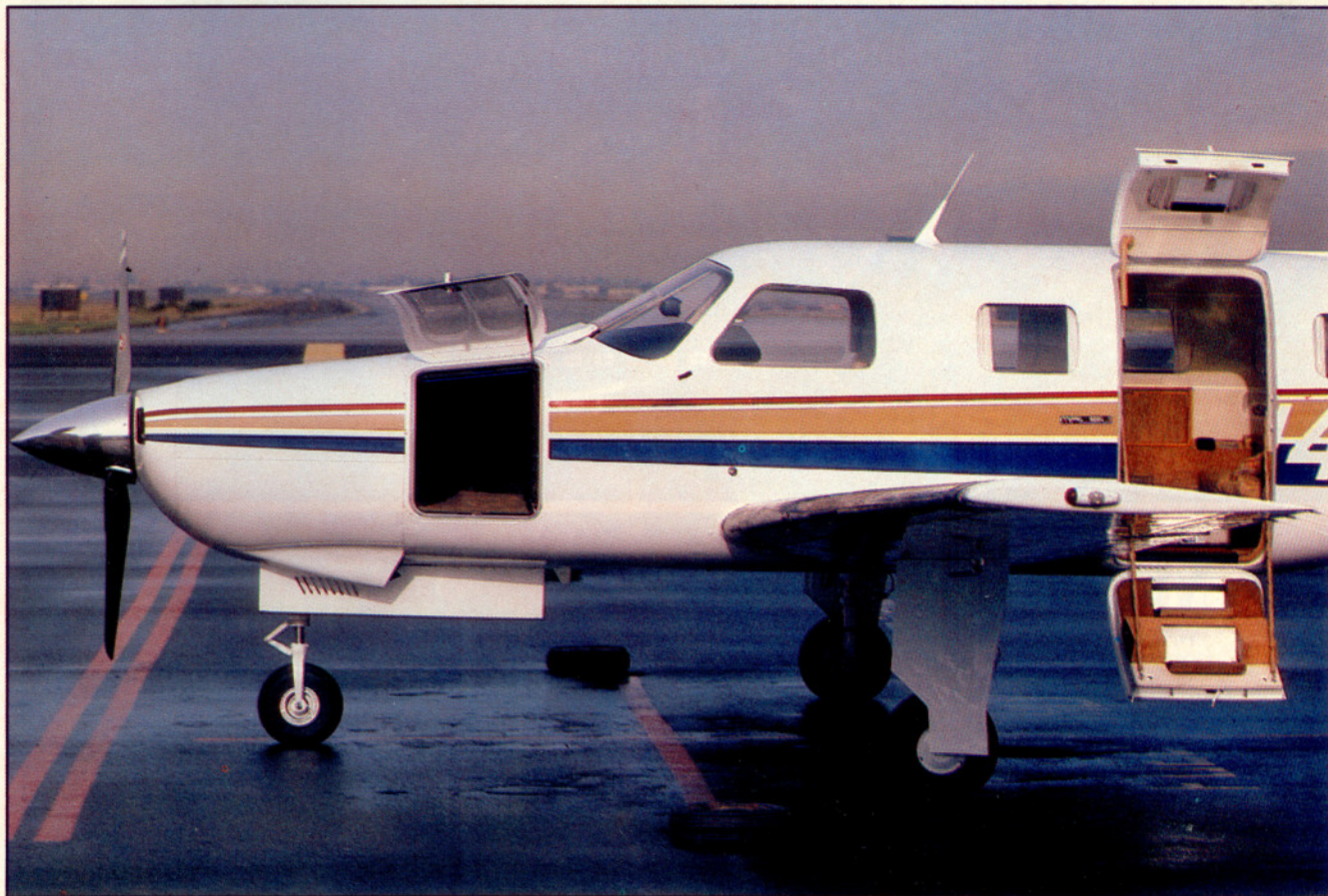
Opened up, the good access to baggage and people space is obvious. The forward baggage compartment helps isolate the pressure vessel from noise, heat and vibration. It helps pilots balance loads. The clam shell air stair door's steps deploy automatically.
